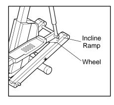
ramp where the wheels make contact with it. Other parts of the elliptical crosstrainer can also be cleaned in this manner. **Never use abrasives or solvents.**
